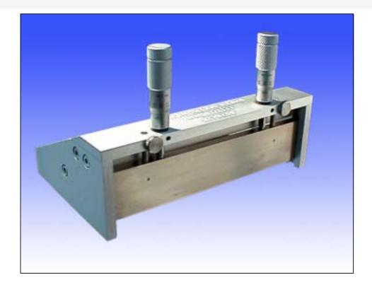
Wet film applicator with two built-in metric micrometer heads for adjusting the knife blade so that clearances of the blade can be accurately set from 0-8mm in 10 micron (0.01 mm) increments.
